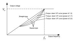
The VFD also provides multi-point V/F curves. You can change the V/F curves output by the VFD by setting the voltage and frequency of the three points in the middle. A whole curve consists of five points starting from (0Hz, 0V) and ending at (motor fundamental frequency, motor rated voltage). During setting, follow the rule:  $0 \le f1 \le f2 \le f3 \le Motor$  fundamental frequency, and,  $0 \le V1 \le V2 \le V3 \le Motor$  rated voltage
