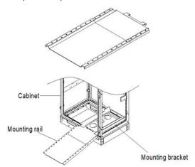
Figure 4-14 Mounting rail diagram
