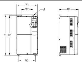
Figure C-6 380V 55-90kW VFD wall-mounting diagram
