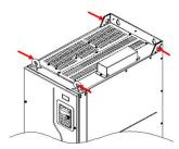
(4) If you need to place the VFD vertically, avoid applying force to VFD sides or placing the VFD on a tilted surface. If the tilted angle is more than 5°, the VFD may suffer rollover since the VFD has a large size and heavy weight (about 200kg).
