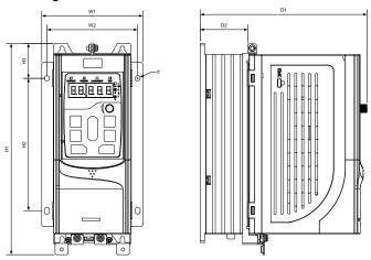
Figure C-10 380V 1.5–7.5kW VFD flange mounting diagram
