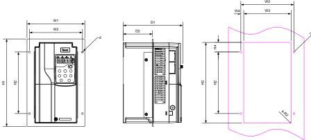
Figure C-11 380V 11- 22kW VFD flange mounting diagram
