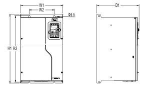
Figure C-7 380V 110-132kW VFD wall-mounting diagram
