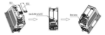
Figure A-1 1.5-7.5kW VFDs with expansion cards installed
