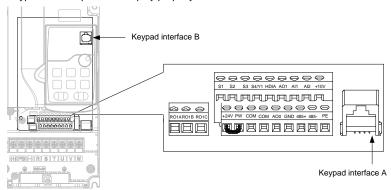
Figure 4-39 External keypad interface
