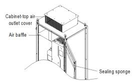
Figure 4-8 Diagram of air baffle design
