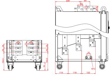
Figure 4-28 Main circuit terminal diagram for 3PH 380V 220–250kW standard models and (-L1) models with built-in DC reactors (unit: mm)
