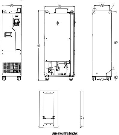
Figure C-14 380V 220-500kW VFD floor mounting diagram
