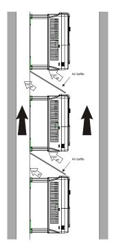
Figure 4-5 Vertical installation
