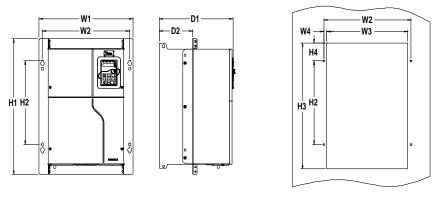
Figure C-13 380V 110–200kW VFD flange mounting diagram
