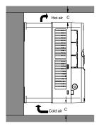
Figure 4-3 Installing one VFD
