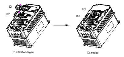
Figure A-2 11-500kW VFDs with expansion cards installed
