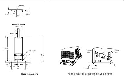
Figure C-16 380V 220-500kW VFD base bracket dimensions and mounting dimensions
