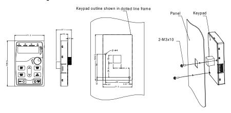
Dimension and hole sizes for mounting keypad without a bracket
