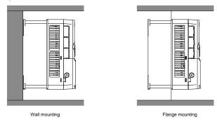
Figure 4-2 Mounting method
