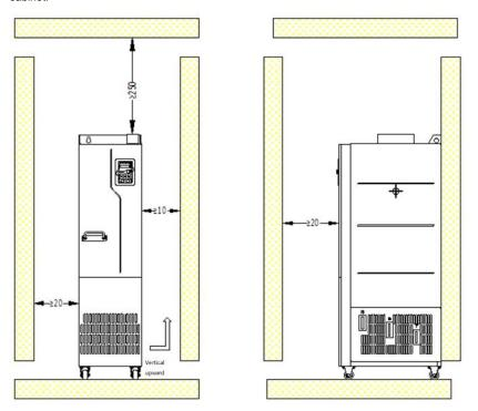
Figure 4-9 Mounting space requirements
