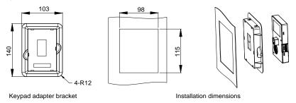
Figure C-2 (Optional) Keypad mounting bracket
