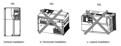
Figure 4-1 VFD installation direction
