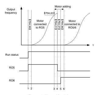
Figure 5-10 Motor adding timing
