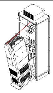
Figure 4-16 Pushing the VFD into the cabinet slowly
