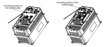
Figure A-4 Expansion card grounding cable connection
