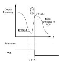
Figure 5-11 Motor reducing timing
