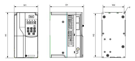
Figure C-5 11–45kW VFD wall-mounting diagram
