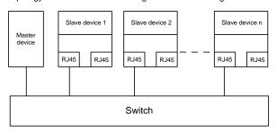
Figure A-8 Star network topology electrical connection
