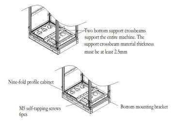
Figure 4-13 Bottom bracket mounting diagram
