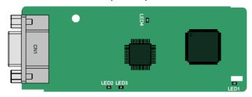
CN1 is a 9-pin D-type connector, as shown in the following figure.
