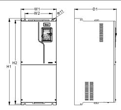
Figure C-8 380V 160-200kW VFD wall-mounting diagram
