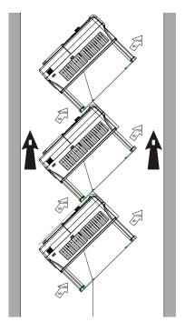
Figure 4-6 Tilted installation
