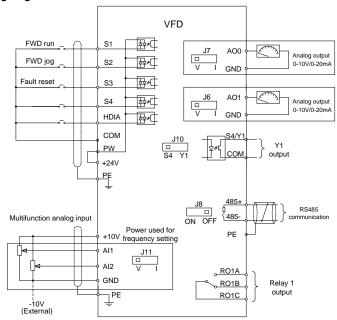
Figure 4-35 Control circuit wiring diagram
