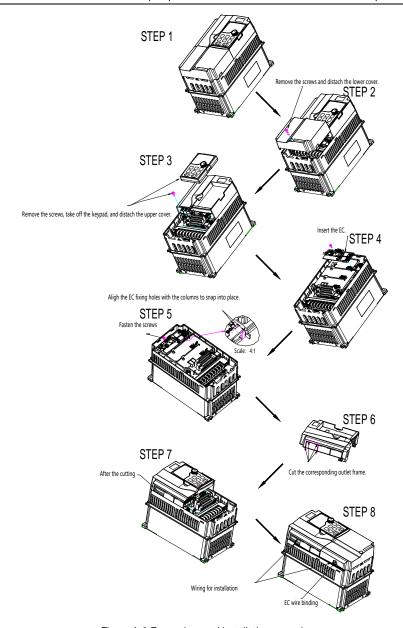
Figure A-3 Expansion card installation procedure
