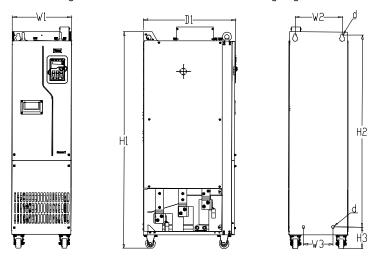
Figure C-9 380V 220-250kW VFD wall-mounting diagram
