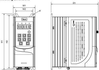
Figure C-4 1.5–7.5kW VFD wall-mounting diagram
