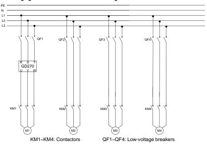
M1-M4: Asynchronous motors
