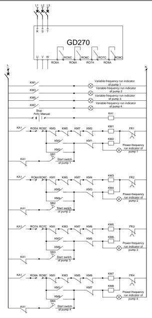
Figure 5-9 External relay control wiring
