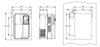
Figure C-12 380V 30-90kW VFD flange mounting diagram
