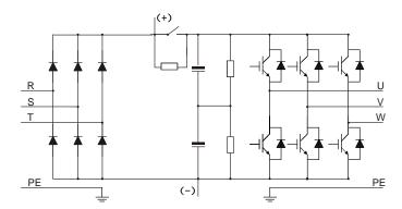
Figure 3-1 Main circuit diagram
