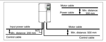
Figure D-3 Cable routing distance
