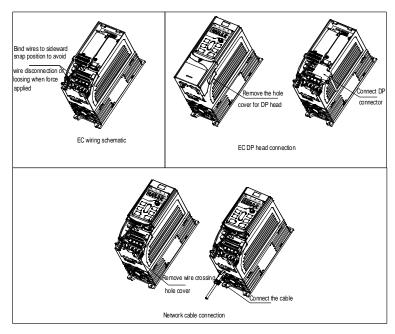
Figure A-5 Expansion card wiring for 1.5-7.5kW VFDs
