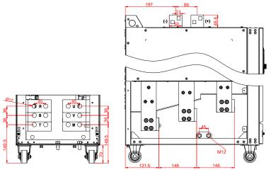
Figure 4-32 Main circuit terminal diagram for 3PH 380V 400–500kW standard models and (-L1)
