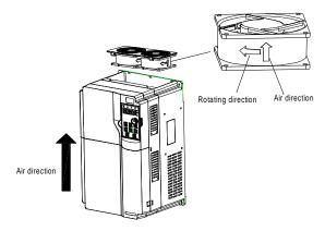
Figure 8-2 Fan maintenance for 11–200kW VFD models
