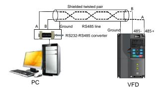
Figure 9-1 Wiring of one RS485 VFD application
