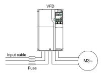
Figure 4-40 Fuse configuration
